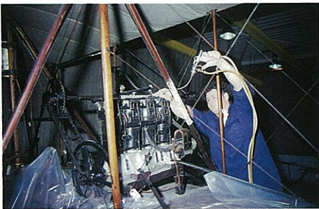
Technical staff at AeroSpace Technology of Australia conserving metal components of the Duigan Biplane PHOTO: Courtesy Museum of Victoria
